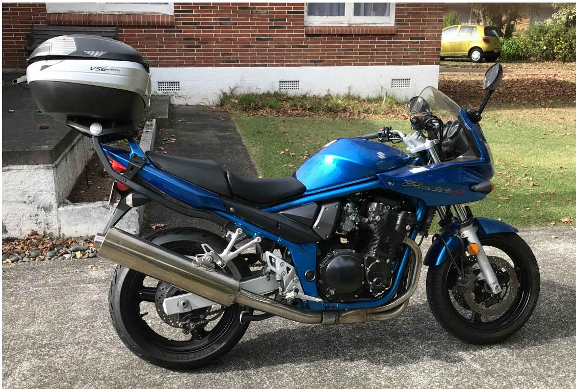
Suzuki GSF 650 S Bandit 656cc 4 cylinder 77 hp @ 10500 rpm bike weight 204 kg dry
