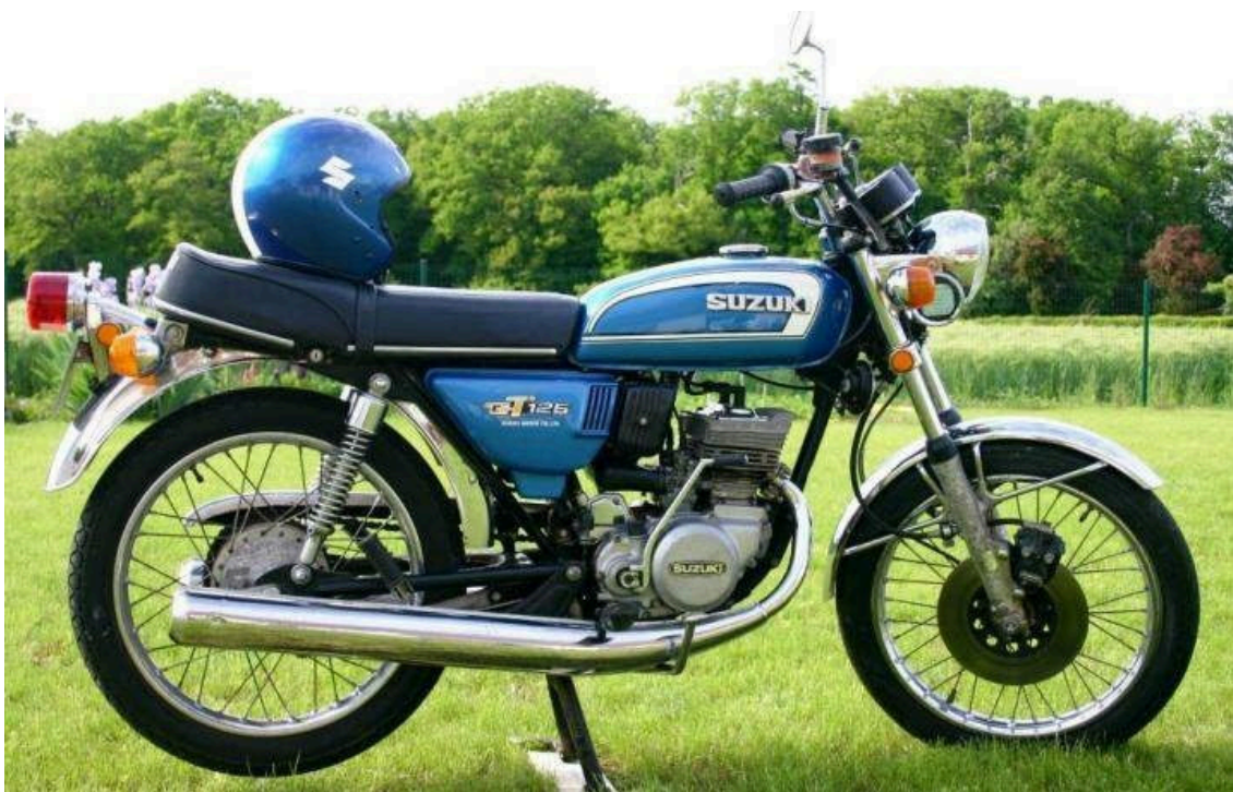
Suzuki GT 125, 1974-77 125cc 2 cylinder 2 stroke 14.2 hp @ 7500 rpm bike weight 115 kg.
