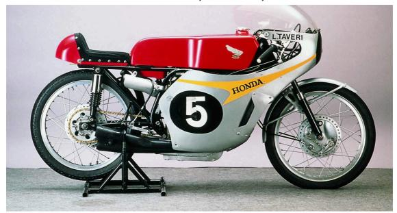
In 1961, 1962 and 1964, Honda four-strokes won three 125cc world titles. But by the middle 1960s two-strokes had evolved into an undeniable force. Debates surrounding engine design had real merit: In a two-stroke engine, every crankshaft rotation yields a power stroke, while four-strokes produce power only upon every other crankshaft rotation—one rotation is "wasted" pushing out gasses. There is no shortcut here; to produce equal power in a four-stroke, engine speeds must increase substantially.
